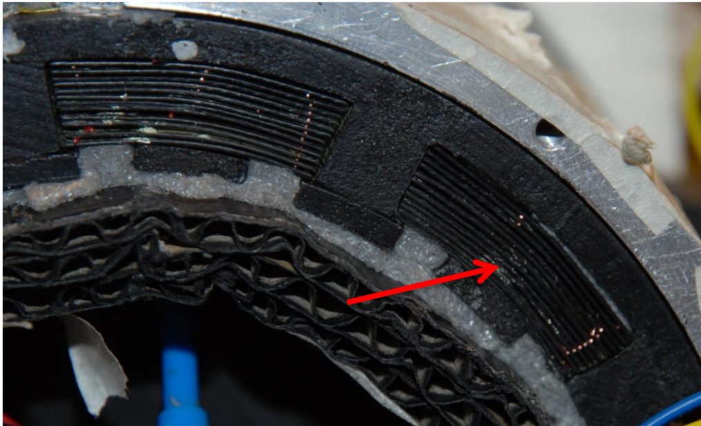
Fig. 5.5.2. Illustration of the layer spacing in prototype machine M1.
